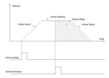
Figure 36: Home to Sensor Profile (Specified Offset)
